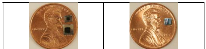
Fig. 1. (Top) Schematic of fuel cell. (Bottom left) Fuel cells of 1 and 4 mm 2 . (Bottom right) H 2 generator integrated with the fuel cell.
