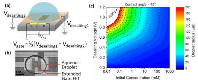
Figure 1. Schematic of (a) FET biosensor with on-chip desalting, (b) image of an extended gate FET with patterned on-chip Pt electrodes and (c) plot of the largest droplet radius ( $\mu\text{m}$ ) that can be depleted using  $10^4 \mu\text{m}^2$  electrodes
