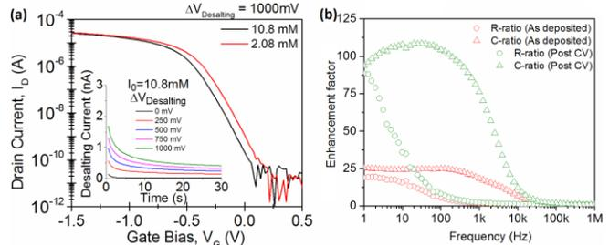
Figure 2. (a)  $I_D$ - $V_G$  sweeps with on-chip gate bias while depleting 500 pL droplet at 1 V desalting bias. Inset shows desalting current in a 10.8mM droplet. (b) Net area increase with Pt-black electrode and CV-treatment through R/C-scaling from EIS shows 100X increase over smooth Pt at low- $f$ .
